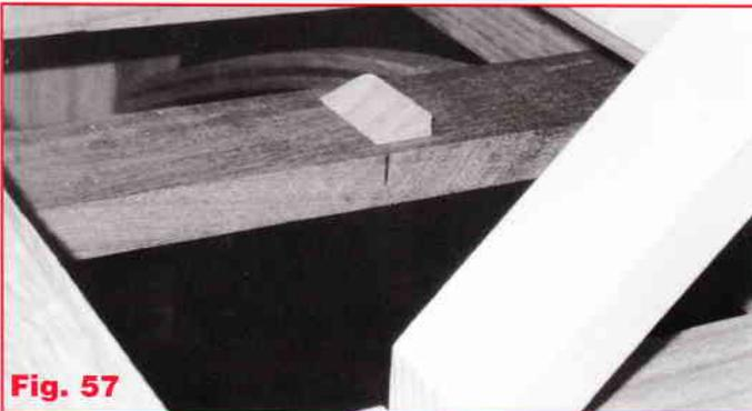
When it is dry, lower the trestle and writing slope and check that when the push rail is pushed in, the wedge raises the writing slope enough for it to be lifted by the finger lifter.
