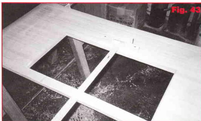
**23** Cut the push rail (**P**) to length from jarrah and shape the front end. Use a rounding over bit in the Router Table (**Fig. 44**).
