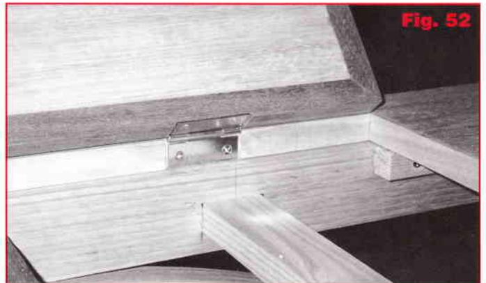
Remove the waste with a sharp chisel and screw the hinges in place (**Fig. 52**).
