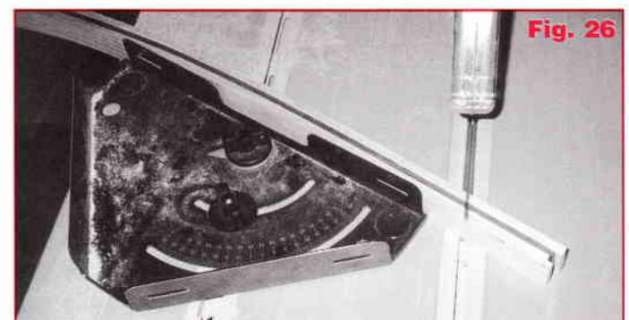
Drill a clearance hole in the centre of the curved rail and a pilot hole in the front rail, then glue and screw it to the desk frame using one 8G x 30 mm screw (**Fig. 27**).
