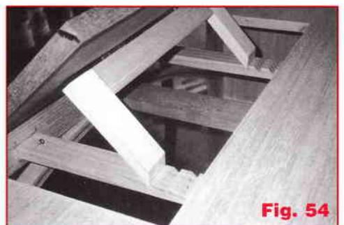
**29** A small wedge (U) is glued to the top of the push rail and rests against the closed trestle. Its job is to push the trestle and writing slope upwards when the push rail is pushed in. It needs to lift the writing slope high enough so the rear of it can be lifted with the finger lifter slot.
