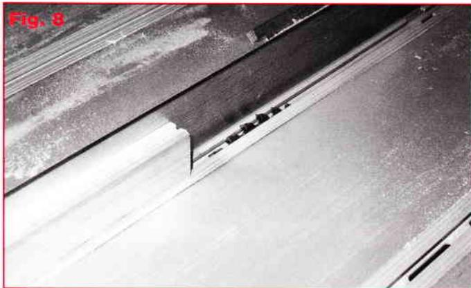
**6** Cut the same sort of rebates in the legs but this time the rebates should stop at the biscuit joints.
