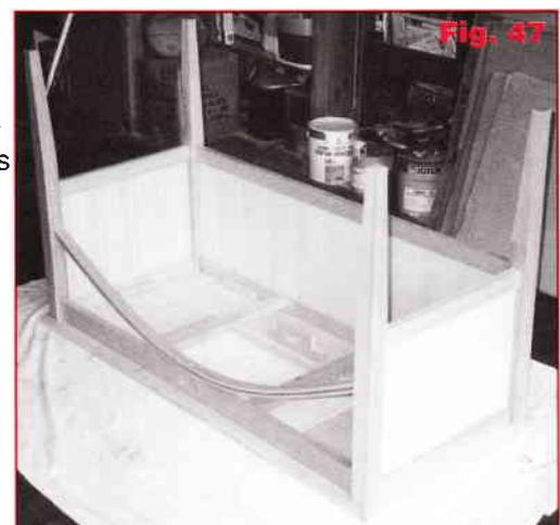
**25** With the desk still upside down, insert the push rail through the slot in the front rail and through the slot in the location block.
